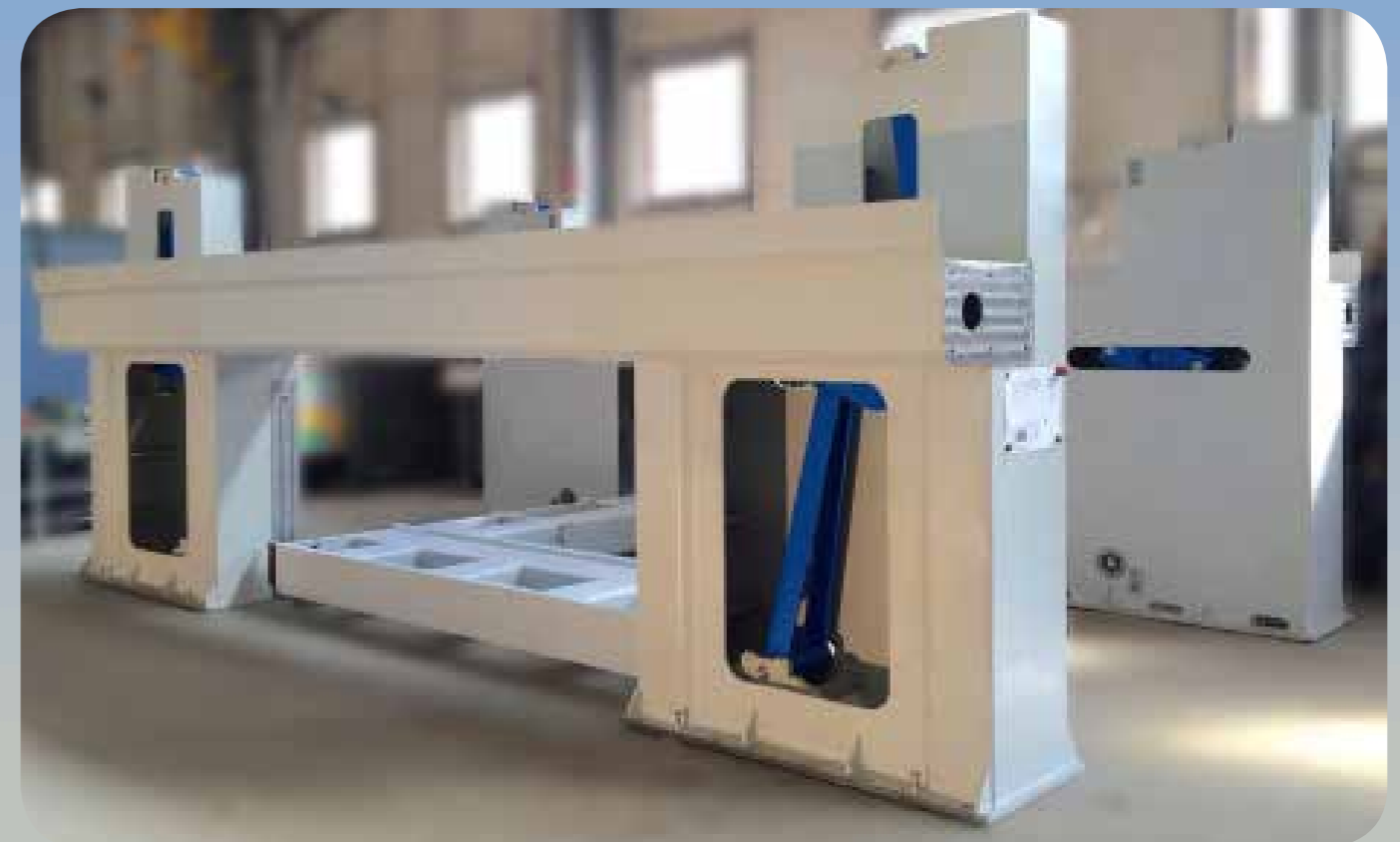
PRIMO TELAIO IN ALLESTIMENTO FIRST GANG SAW UNDER COSTRUCTION
